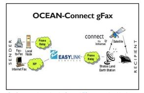
Our fax server, located at the Stratos LES, contacts the ship via satellite, therefore delivering the message quickly, while maintaining a high quality connection. Using OCEAN-Connect gFax provides better control of your fax message transmission and costs.
